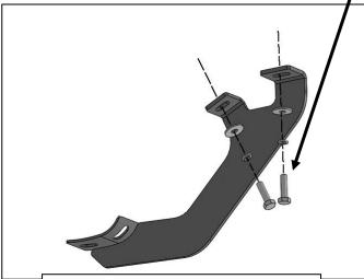
(Fig 2) Attach the Passenger/Right Front Mounting Bracket to the front
