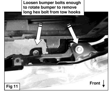
Mounting holes in end of frame for tow hook
