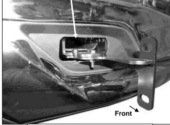
(Fig 19) Driver side Bracket Installed
