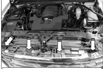
(Fig 2) Remove cover between radiator and grille. Remove screws attaching top of grille (arrows)
