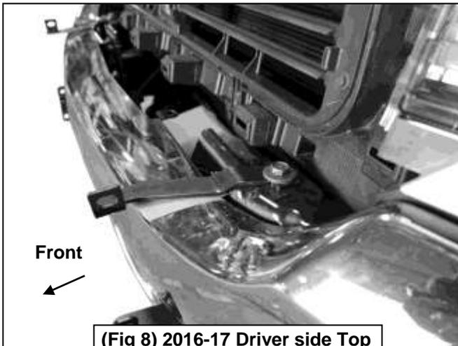
(Fig 8) 2016-17 Driver side Top Mounting Bracket installed
