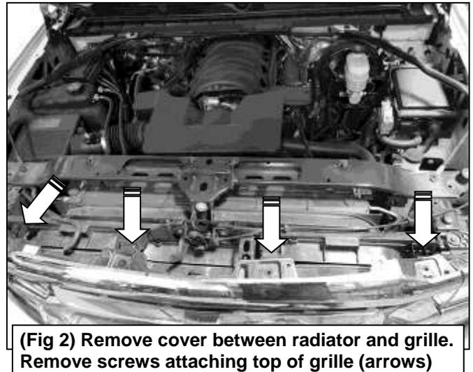
**(Fig 2)** Remove cover between radiator and grille. Remove screws attaching top of grille (arrows)
