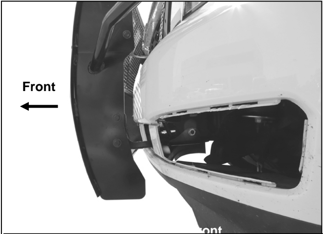
(Fig 21) Attach Grille Guard to Mounting Brackets
