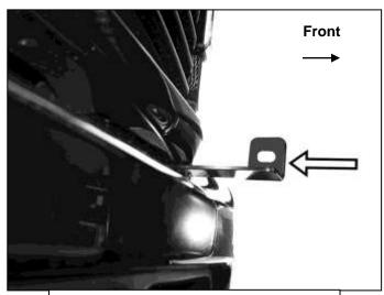
(Fig 4) Insert flat end of driver/left Top Bracket through bumper (arrow)
