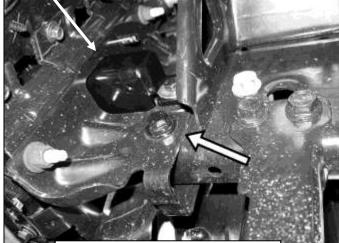
(Fig 10) Remove hex bolt (arrow)
