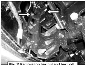
(Fig 1) Remove top hex nut and hex bolt from back of bumper bracket (arrows).
