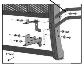
(Fig 13) Attach Grill Guard to outside of driver/left Mounting Brackets
