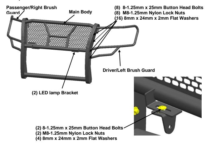
IMPORTANT: The Grille Guard is designed to tilt forward to clear the attached grille on 2007-13 Tundra, 08-14 Sequoia models. To tilt the Grille Guard, the Quick Release Bolts on the Top Brackets must be released and the upper bolts on both Mounting Brackets may need to be loosened slightly. Make sure that all hardware is fully tightened after closing the hood. Carefully read Page 8, "Opening and Closing of Hood," before installing the Grille Guard.
