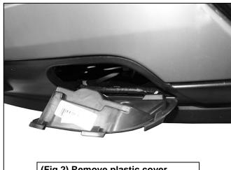
(Fig 2) Remove plastic cover (model without tow hook pictured)
