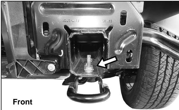
**(Fig 8) Temporarily remove tow hooks if equipped**
