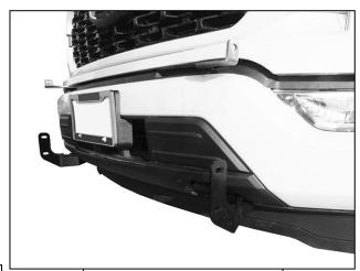
(Fig 13) Brackets installed
