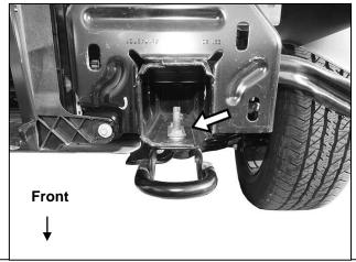
(Fig 8) Temporarily remove tow hooks if equipped
