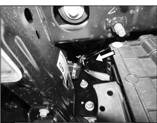
(Fig 3) Unplug all wiring harnesses leading to the front bumper (arrow)
