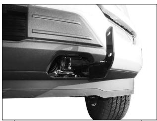
(Fig 12) Driver/left side Mounting Bracket installed without tow hook
