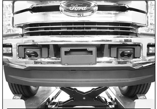
(Fig 6) Remove plastic air dam from bumper
