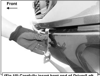
(Fig 10) Carefully insert bent end of Driver/Left Support Bracket through gap between lower bumper and upper plastic fascia panel. Use removable tape to protect finish on bumper
