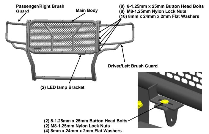
IMPORTANT: The Grille Guard is designed to tilt forward to clear the attached grille on 2007-13 Tundra, 08-14 Sequoia models. To tilt the Grille Guard, the Quick Release Bolts on the Top Brackets must be released and the upper bolts on both Mounting Brackets may need to be loosened slightly. Make sure that all hardware is fully tightened after closing the hood. Carefully read Page 8, "Opening and Closing of Hood," before installing the Grille Guard.
