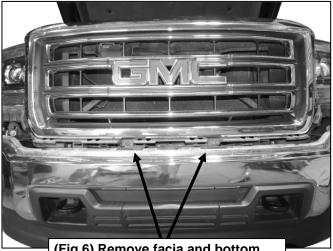
(Fig 6) Remove facia and bottom bolts attaching grille to the vehicle
