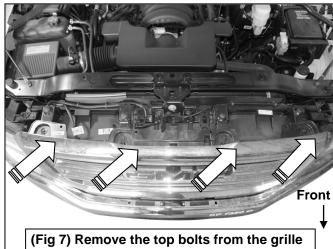
(Fig 7) Remove the top bolts from the grille and carefully pull and remove grille
