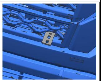
(Fig 4) Attach Driver/Left Inner Support Bracket to vehicle
