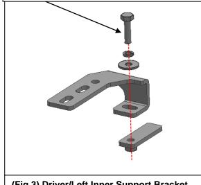
(Fig 3) Driver/Left Inner Support Bracket installed.
