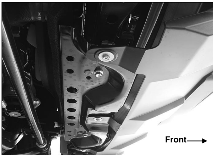
(Fig 2 ) If necessary, temporarily remove bumper cover hardware to access bumper bracket (passenger/right side pictured from below)
