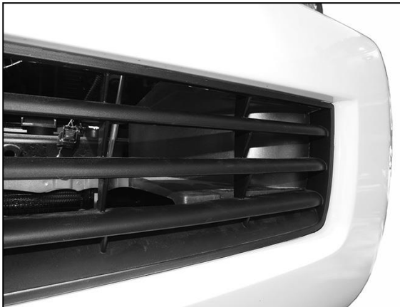
(Fig 5A) Remove or cut air deflector from behind lower grille opening in bumper
