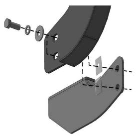
Insert a Plastic Washer between the Grille Guard and the Frame Mounting Bracket on each 12mm Hex Bolt
