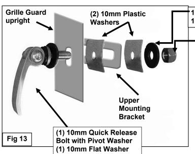
10mm Flat Washer 10mm Nylon Lock Nut
