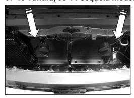
Upper Mounting Bracket Adapter Plates must be installed on the frame from above
