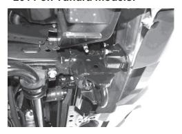
Upper Mounting Bracket Adapter Plates must be installed on the frame from below the front bumper.
