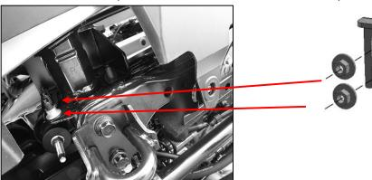
Slide the Bracket over the two threaded studs.( If installing from below, carefully pull the bottom of the bumper cover outward and slide the Bracket up and in position). Reuse the factory hex nuts to attach the Bracket to the frame. Do not fully tighten the (2) hex nuts at this time.
