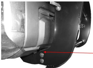
Loosen the Upper bolts (only if necessary) to open the hood.
