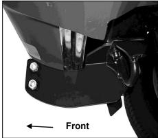
Mounting bracket uses the factory tow hook mounting bolts. Small tow hook (pictured) can be re-installed, the larger tow-hooks cannot. Repeat process to install Driver's(left) Side
