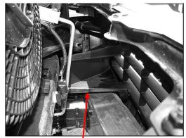
Some models have an air deflector mounted on the driver's side, it may be necessary to remove the bumper cover to trim or remove this.
