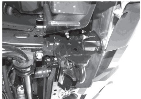
Upper Mounting Bracket Adapter Plates must be installed on the frame from below the front bumper.
