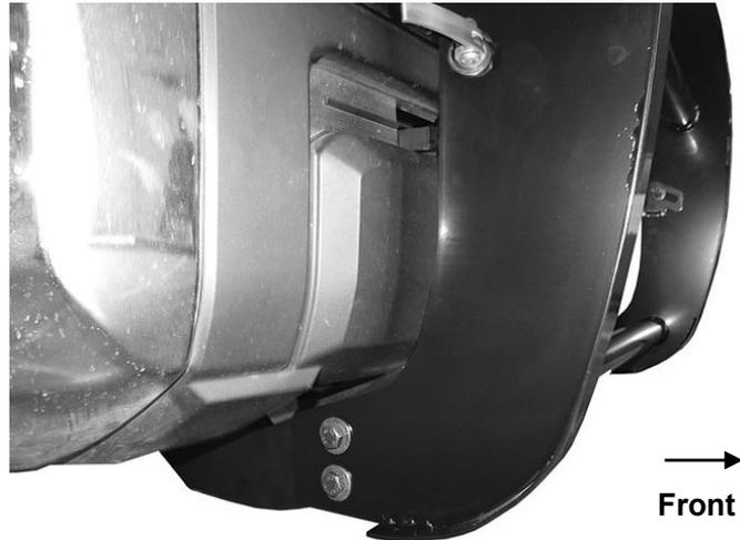
Insert a Plastic Washer between the Grille Guard and the Frame Mounting Bracket on each 12mm Hex Bolt
