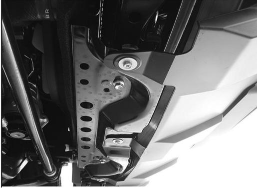
If necessary, temporarily remove bumper cover hardware to access bumper bracket. (passenger/right side pictured from below)
