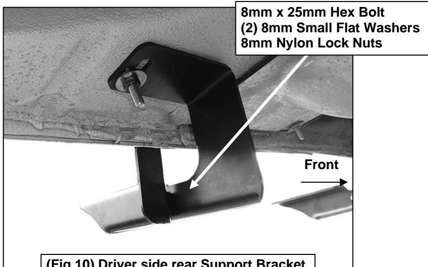
(Fig 10) Driver side rear Support Bracket
