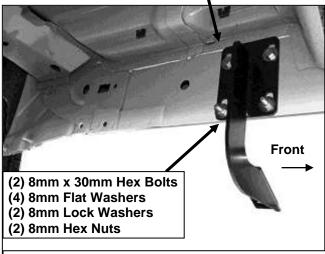
(Fig 5) Passenger/right front Bracket installation pictured
