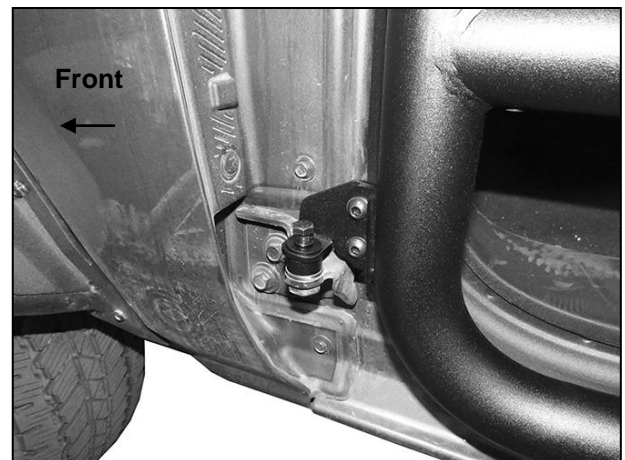
(Fig 18) Tighten hardware on Hinges (driver/left Lower Hinge pictured)
