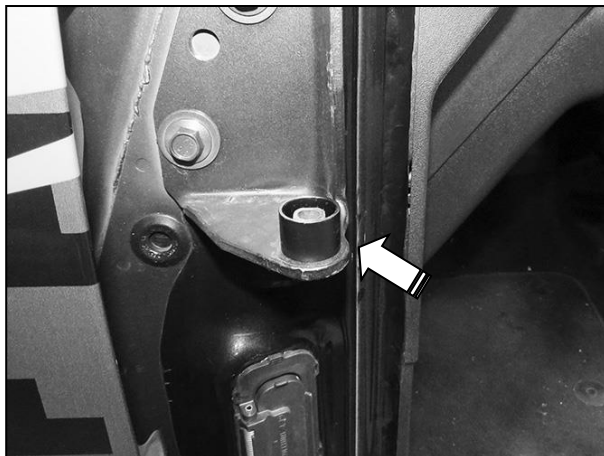
(Fig 8) Slide Tall Nylon Upper Tube Spacer onto hinge post (arrow)
