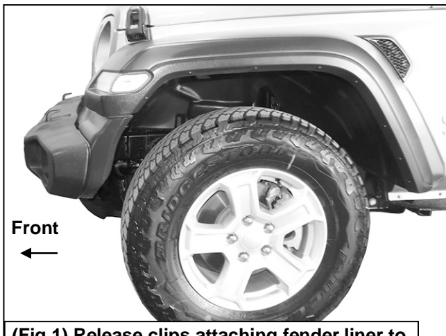
(Fig 1) Release clips attaching fender liner to outer fender
