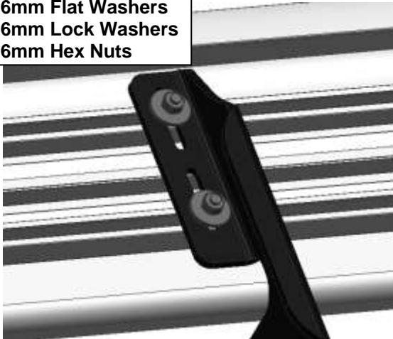
(Fig 13) Attach Running Board to Brackets
