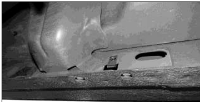
(Fig 4) Passenger/right front or rear Bracket attached to pinch weld
