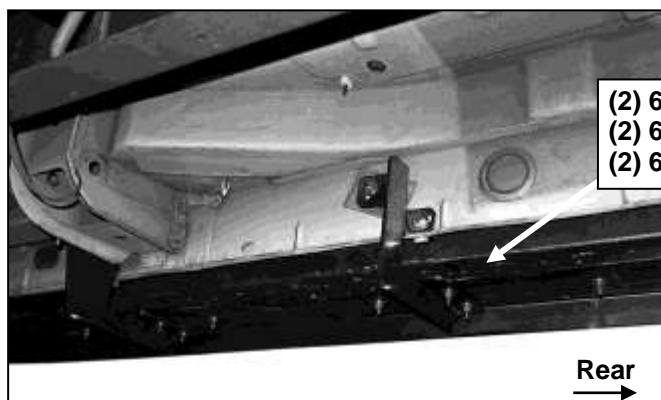
(Fig 32) Passenger/right #3 Bracket installation
