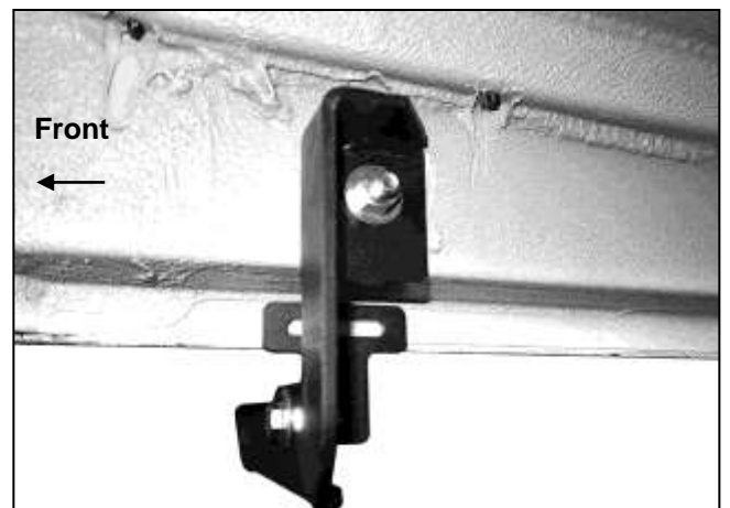
(Fig 6) Passenger/right Front Bracket installed
