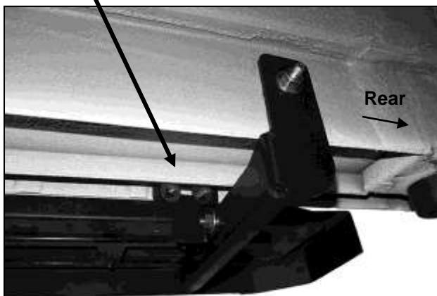
(Fig 15) Attach Support Bracket to pinch weld (passenger/right rear Bracket pictured)
