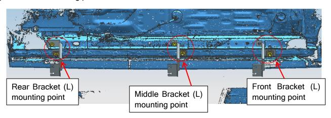
Step 2: Attach Front Bracket (L) ①, Middle Bracket (L) ③ and Rear Bracket (L) ⑤ on the mounting points with T Bolts M10x40⑦, Plastic Retainers $\phi$ 10 ( $\delta$ 0.7\*40\*40) ⑧, Hex Nuts M10⑨, Flat Washers D10 (10x30x2.5mm) ②, Flat Washers D8 (8x24x2mm) ①, Hex Bolts M8\_30①, Lock Washers D8① and Lock Washers D10①4. Front Bracket (R)②, Middle Bracket (R)④ and Rear Bracket (R)⑥ refer to left side installation, and the right and right sides are symmetrical.
