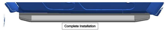
STEP4: After the running boards are adjusted to the appropriate position, lock all the standard parts. The installation position and manner of the left side brackets are the same as that of the right side.
