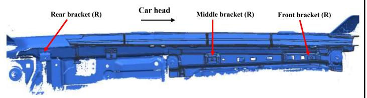
STEP2: Find the corresponding installation position of brackets in the figure (the picture shows the right side of the car).
