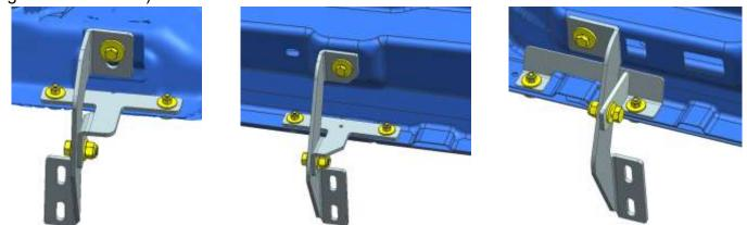
STEP3: Fix the brackets with standard parts according to the assembly diagram (standard parts do not need to be locked at this time).
