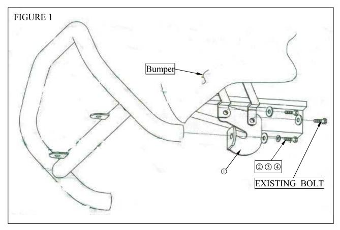
STEP 5. Attach Safari Bar to brackets using 1/2" fasteners. Hand tighten.
