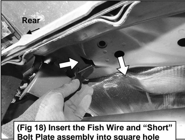
(Fig 18) Insert the Fish Wire and "Short" Bolt Plate assembly into square hole and down through floor (arrow)
