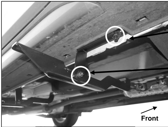
(Fig 7) Passenger side Front Support Bracket installed
