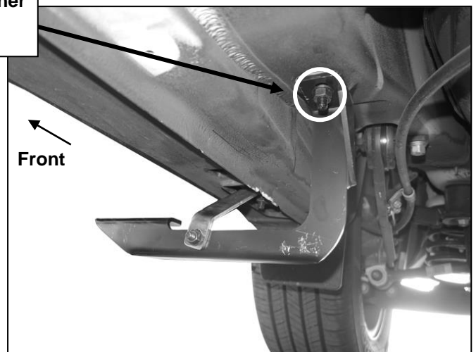
(Fig 10) Passenger side rear bracket installed
