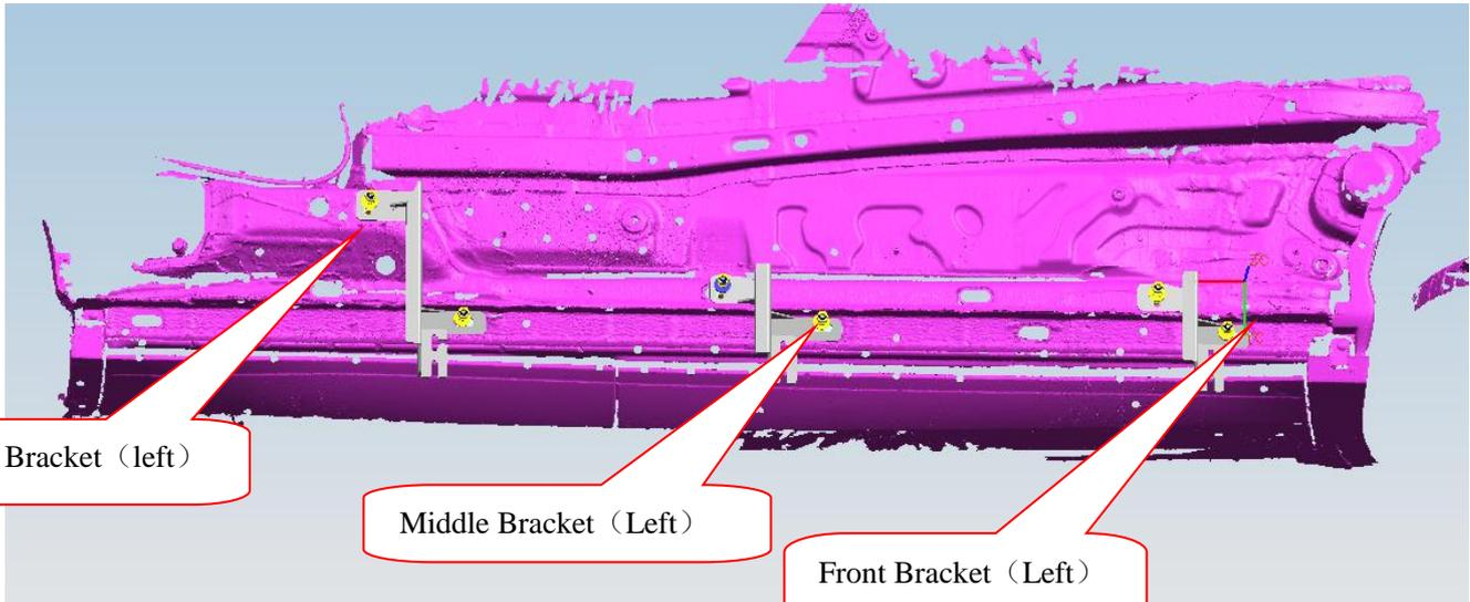
Step 3: Install the side bar on the brackets and then adjust them to the proper positions.
