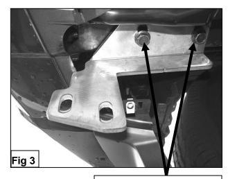
Replace factory bolts with the included: 12-1.25 x 35mm Hex Bolts 12mm Lock Washers 12mm Flat Washers
