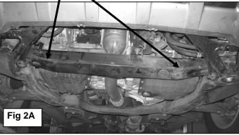
12mm x 100mm Hex Bolt (2) 12mm Flat Washers 12mm Nylon Lock Nut
