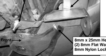
8mm x 25mm Hex Bolt (2) 8mm Flat Washers 8mm Nylon Lock Nut
