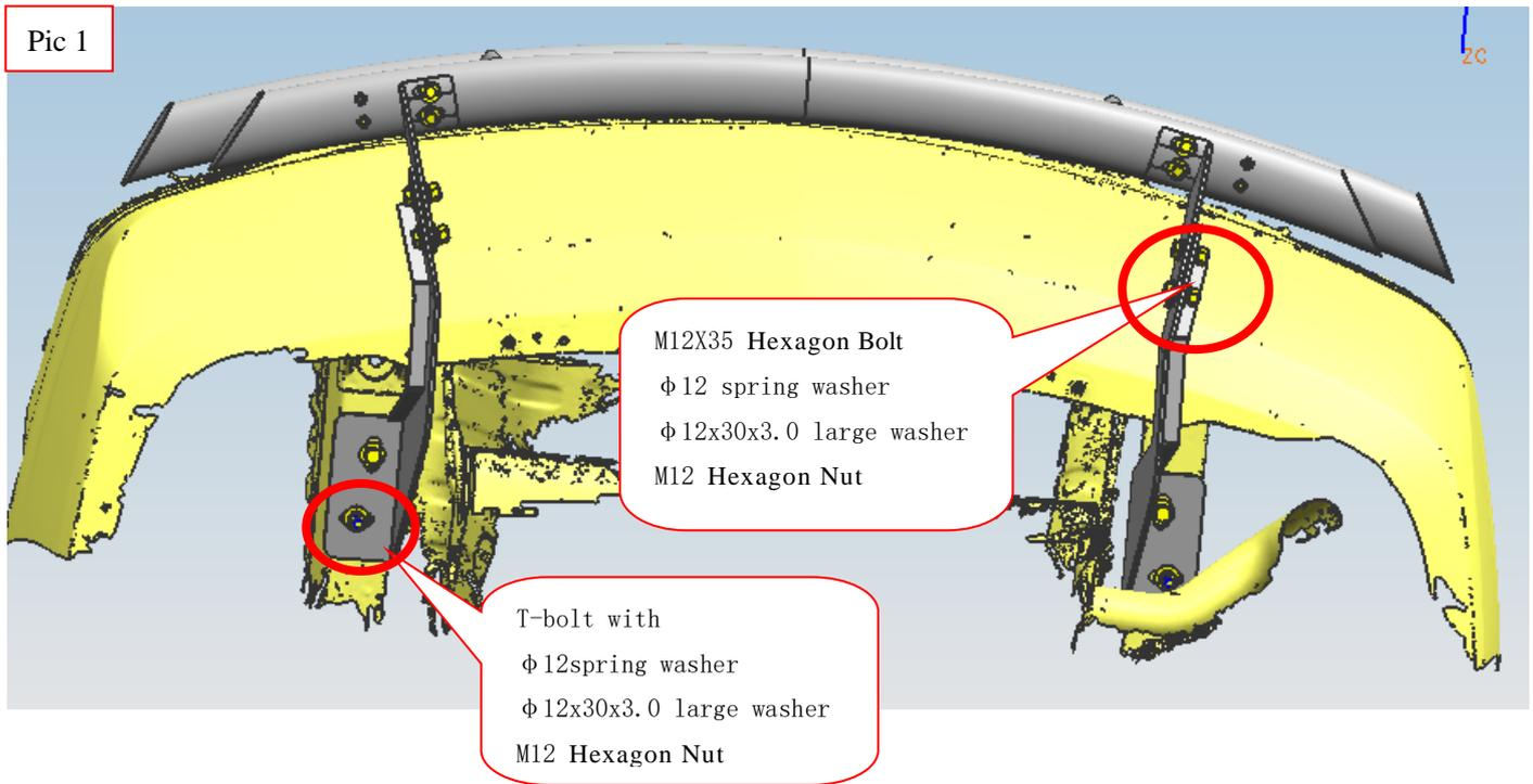
Step 3: install the rear bumper on the brackets and adjust the rear bumper to the proper position.
