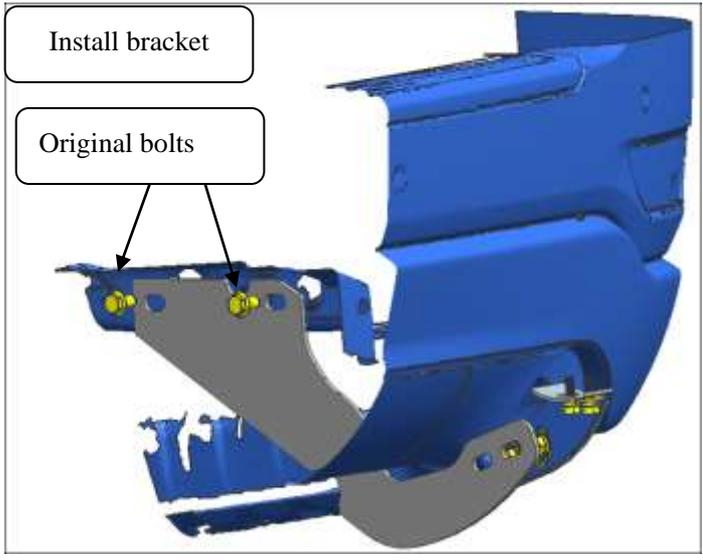
Step 3: Install the bracket-A on the bracket-B by part ⑥⑦⑧⑨, Do not tighten all of them.
