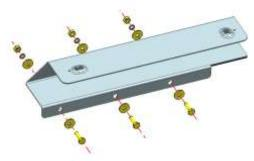
Step 6: Install the roll bar, mounting base and roll bar gum covers with standard part 39
