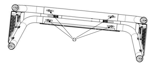
**Step 5:** Put mounting base(L/R) on both sides of the truck rail, to adjust the mounting base on suitable position, then mark down the installation holes for drilling(Ps: To make sure the drilling holes can go through with M10 standard parts). Install the mounting base on truck rail with standard parts (3) (3) (3) (4), as the following picture shown.
