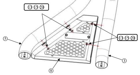
**Step 4:** After the preceding components are preinstalled, connect the side tube and middle tube with standard part ②.(To adjust tubes to appropriate position, lock tighten all accessories except standard part ②) PS: These adjustable holes can control the width of roll bar.
