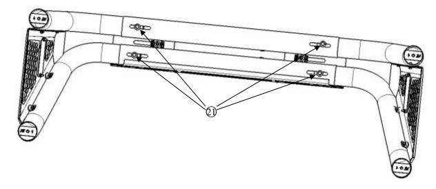
**Step 5**: Slip each 3 pieces T-bolts into both sides of utility side trail as the following picture shown, and put mounting base on the truck rail and adjust base to appropriate position, install them with standard parts 30 3.
