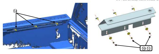
**Step 6:** Put the gum covers on each legs of roll bar, then install roll bar on mounting base with standard part ②. To adjust roll bra to appropriate position and lock tighten all standard parts.
