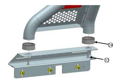
**Step 7**: Install the front and rear end cover with standard part ②.
