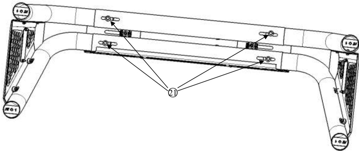
**Step 5:** Slip each 3 pieces T-bolts 34 into both sides of utility side rail as the following picture shown, and put mounting base on the truck rail and adjust base to appropriate position, install them with standard parts 30 31.
