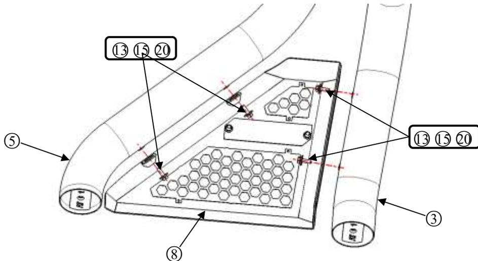
**Step 4:** After the preceding components are preinstalled, connect the side tube and middle tube with standard part 21. (To adjust tubes to appropriate position, lock tighten all accessories except standard part 21) PS: These adjustable holes can control the width of roll bar.
