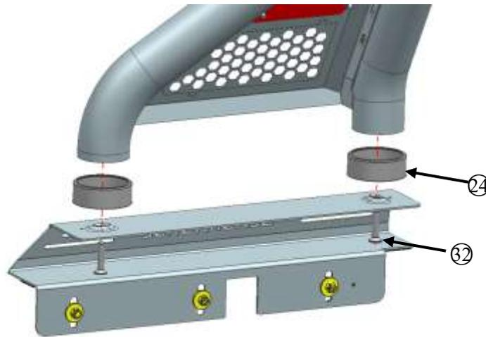
**Step 7:** Install the front and rear end cover with standard part 23.
