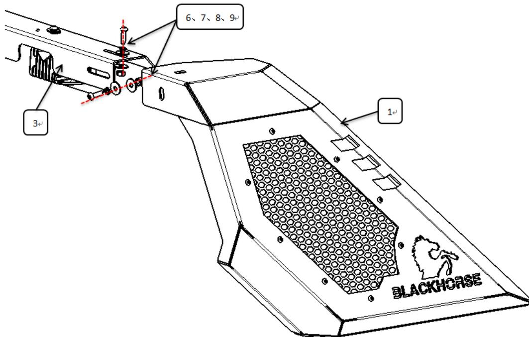
Step 3: Test and make sure that the roll bar is steadily fixed, fully tighten all hardware.
