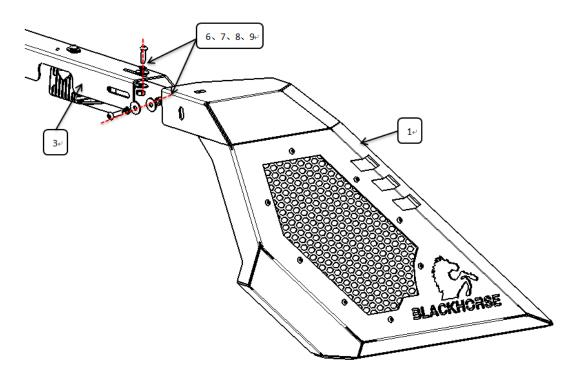
Step 3: Test and make sure that the roll bar is steadily fixed, fully tighten all hardware.
