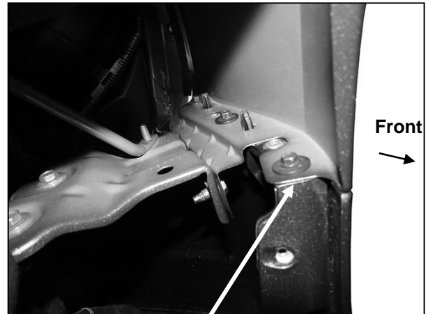
(Fig 6) Remove hardware attaching bumper cover to fender. Remove bumper cover
