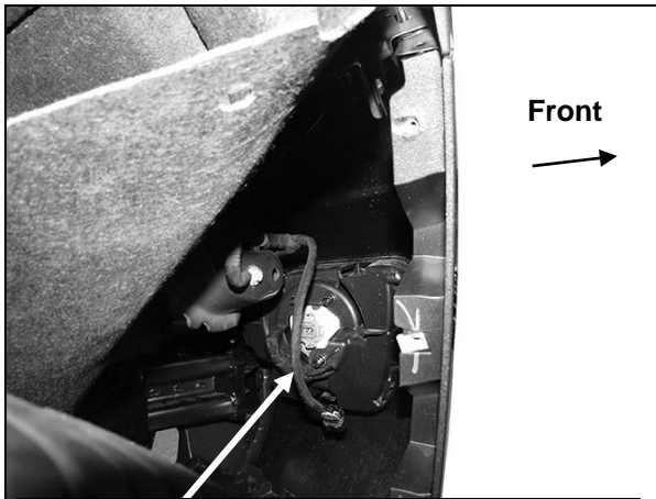
(Fig 7) Pull back fender liner to access bumper hardware and unplug fog light if
