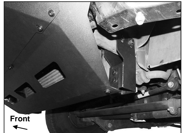
(Fig 30) Skid Plate installed
