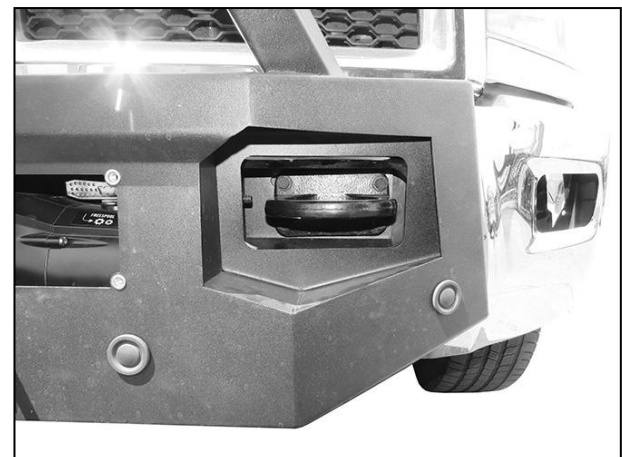
(Fig 24) Bumper installed with tow hook
