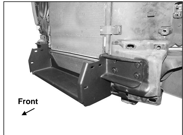
(Fig 9) Winch Tray attached to frame (model without tow hooks)
