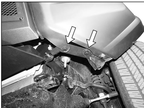
(Fig 20) Driver/left side of bumper cover attached to Support Bracket (arrows)
