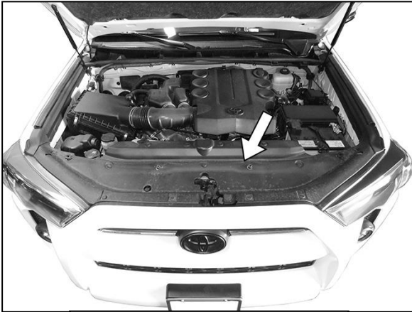
(Fig 3) Remove plastic cover from top of radiator (arrow)
