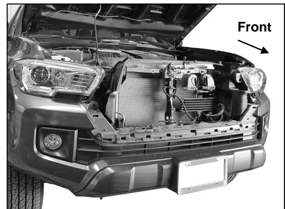
(Fig 2) Remove grille, license plate, bracket and air dam
