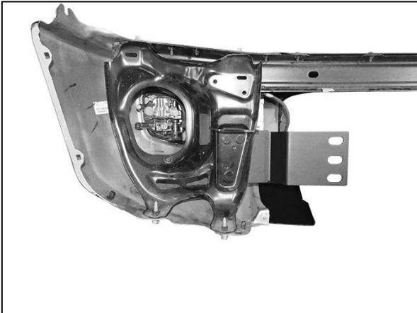
(Fig 18) Reuse the factory hardware to attach the Reinforcement Brackets to the crossbar brackets. Reattach the crossbar brackets and bumper to the side panels
