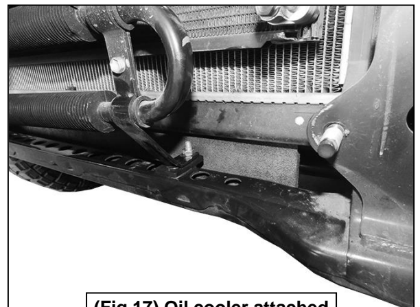
(Fig 17) Oil cooler attached to the Spacer Plate
