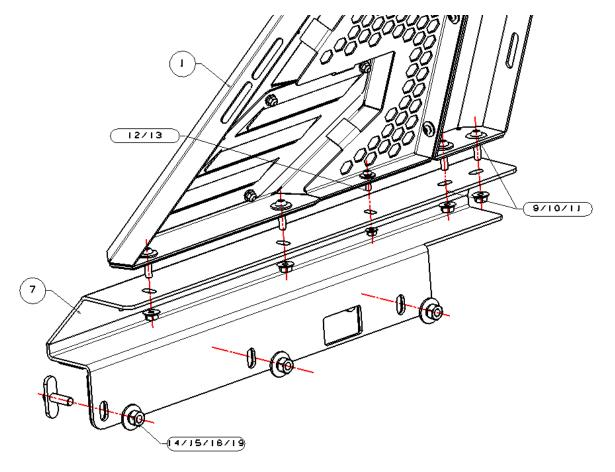
Step 4: Install roll bar on truck rail by hard standard parts 4 15 6
