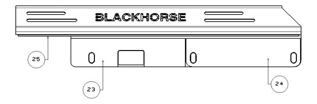
**Step3:** Connect the roll bar with mounting base by the standard parts 9101/1213.
