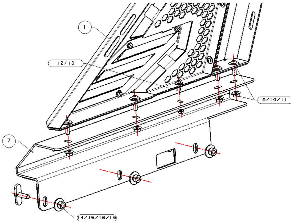
**Step 4:** Install roll bar on truck rail by hard standard parts ⑭ ⑮ ⑯ ⑰
