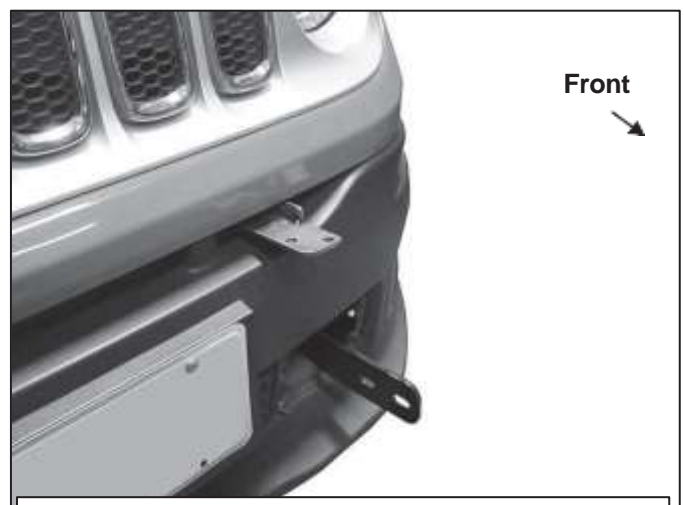
(Fig 17) Before reinstalling the bumper cover/grille, cover edges on brackets with removable tape (masking tape for example). Carefully guide bumper cover/grille assembly over the bumper brackets and back into position.
