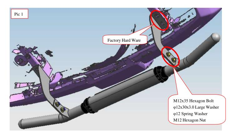
Step 3: Install the rear guard on the brackets and then adjust them to the proper positions.
