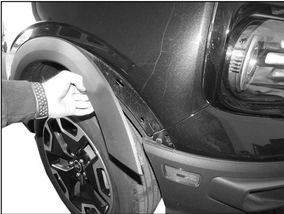
(Fig 5) Firmly pull the front of the fender flare out from the bumper (passenger/right side pictured). Do not remove the flare, only release the front end of the flare
