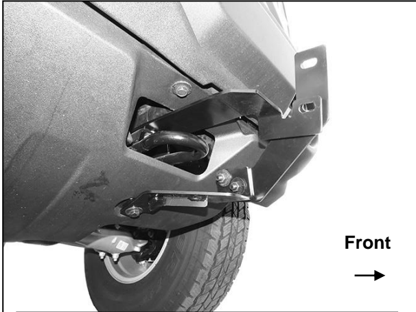
(Fig 11) Driver/left side Brackets installed
