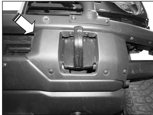
(Fig 6) Model with steel bumper, remove lower splash guard/skid plate and cover around tow hook (driver/left side pictured)
